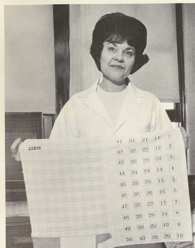
Dr. Laverne Bandy Thomas, associate in detergency research, holds a TWU laundry test assembly designed for measuring soil removal, whiteness retention, and fabric strength preservation.
