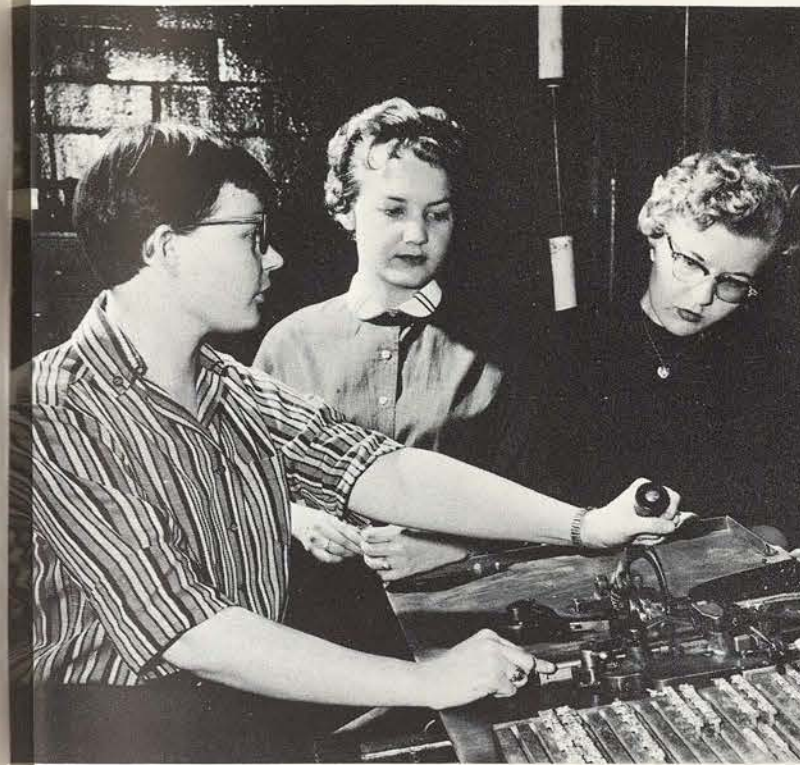
A senior journalism major demonstrates the operation of the Ludlow to two other students. The machine, which sets metal headline type used in the newspaper, is but one of the many pieces of useful and modern equipment found in the journalism building print shop.
