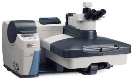
Figure 11. The figure above illustrates the Raman Instrument used throughout the experiment. DXR Raman Microscope with a laser power of 532nm.
