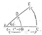
Lever 10 - moves twice as far and twice as fast as lever AB (if-the distance is convered in the same period of time)
