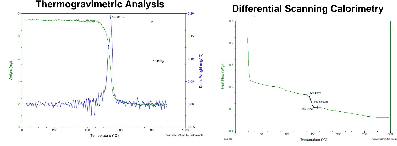
• The infrared, IR, spectrum and the thermal analyses confirm that the main component of our plastic is a polycarbonate polymer.
