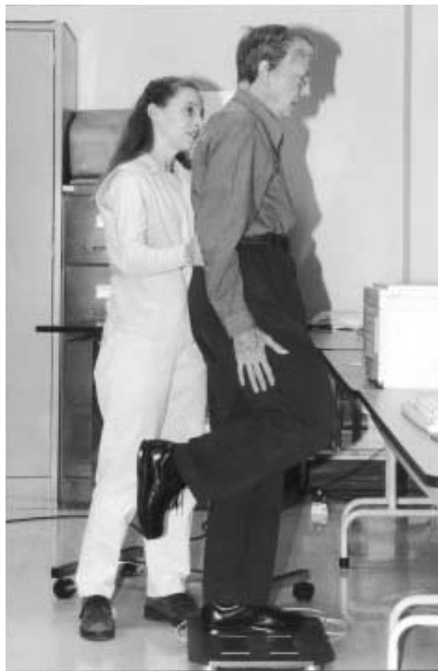
FIGURE. Measures of postural stability in single-stance were obtained using the BEP IV force platform.
