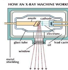
Figure 5: <sup>8</sup>Anodes and cathodes in an x-ray.
